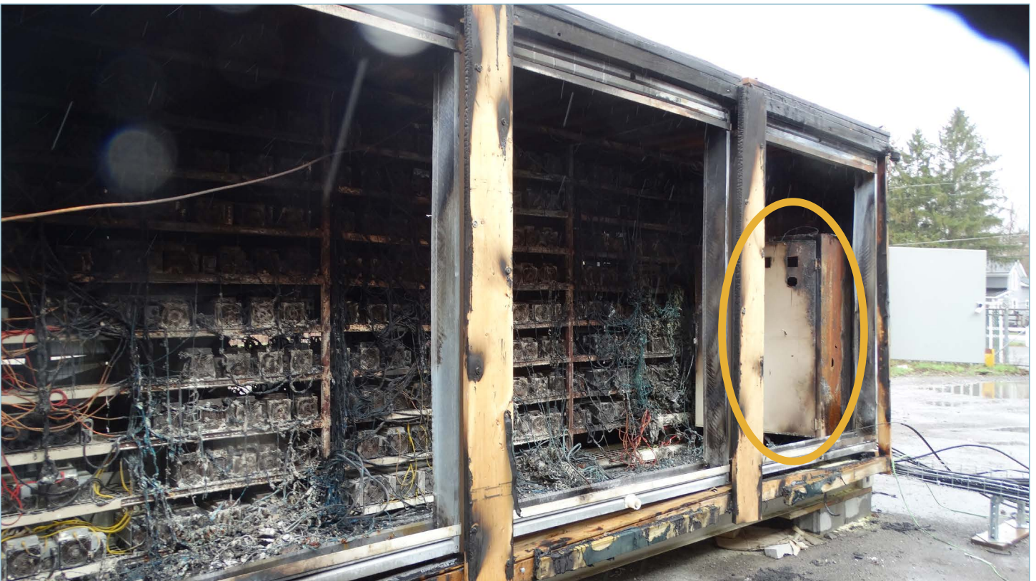
The power distribution panel in the affected container. Picture credit Envista Forensics.
